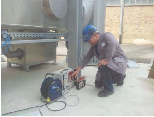
Wash bottle equipment with calibrated measuring gas pump
