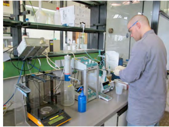
Determination of ammonia by titration
